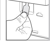
4. pull outwards using the tab as indicated in the figure, until the plastic tie-rod is freed from its stop position; pull downwards and open the door at the same time.5. reposition the panel, making sure the hooks are securely in place before you push it onto the appliance.
